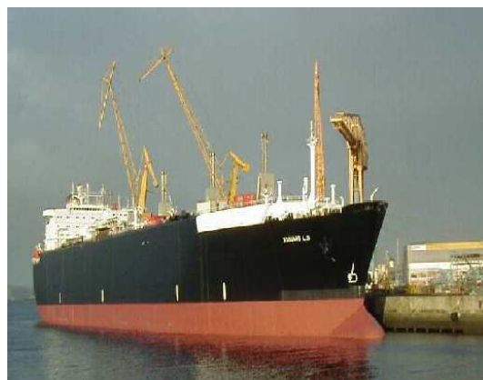
April 05 - EDOUARD L.D. alongside during a 66 days major up-grading work in membrane tanks. Note the special handling protections above tank entries.
